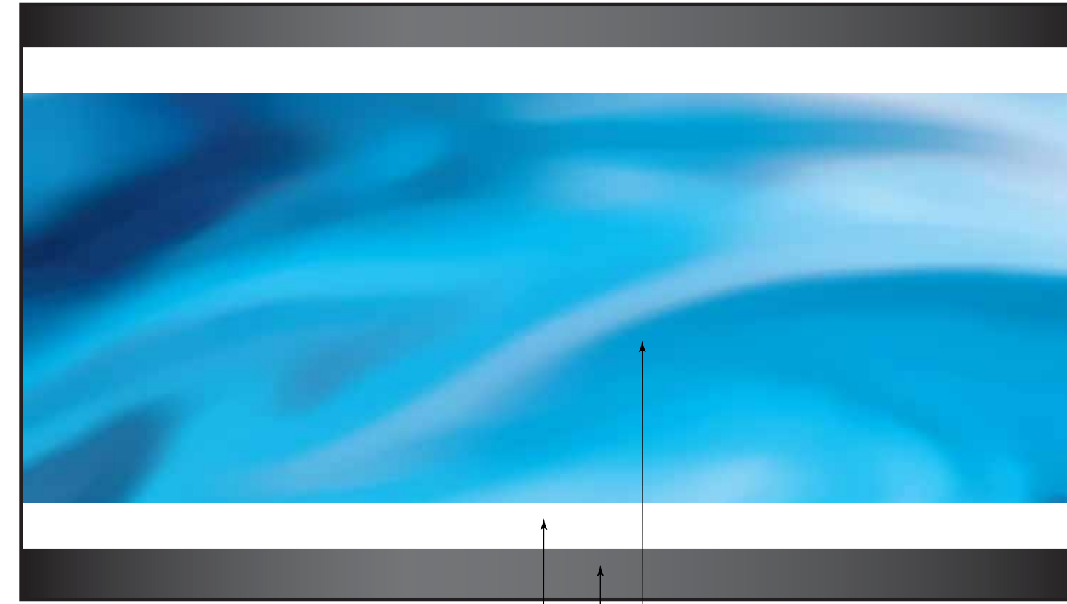
DECORATIVE CROSSWALK_OPTION #2 WHITE AGGREGATE LITHOCRETE | AQUA GLASS LITHOCRETE | EXISTING ASPHALT | SCALE: NTS
